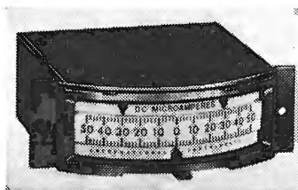
International Instruments indicator-controller. The limits are set by the two pointers over the scale.
