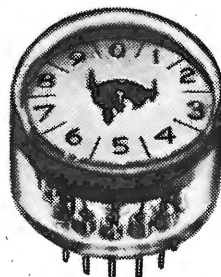
Mullard neon indicator tube for low signal-voltage applications, such as transistor counters.
